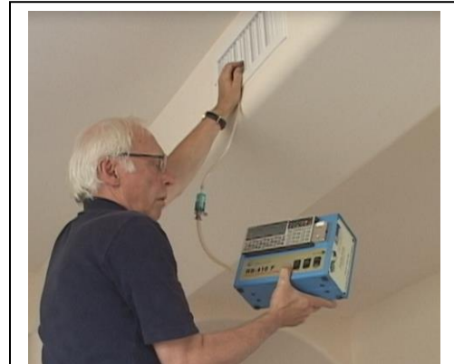
Figure 22: Grab Sampler as Diagnostic Tool
