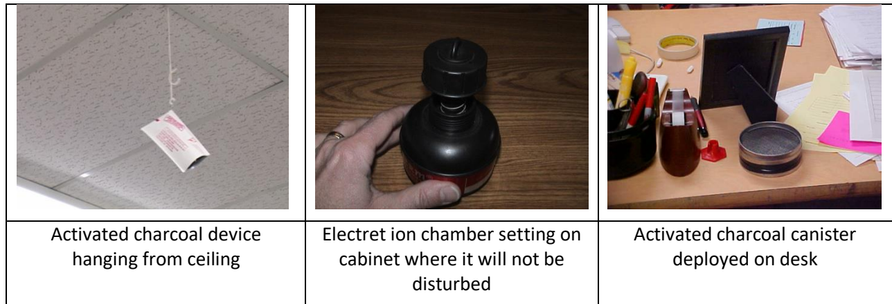
Figure 32: Examples of Common Radon Measurement Devices
